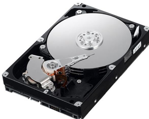
It consists of one or more platters with a special magnetic coating and 1 or more drive heads that skip across the platter(s) reading and writing digital information. Information is stored in cylindrical tracks across the whole drive platters. When you first purchase a computer the operating system has been freshly installed and the files are generally organized in a contiguous block as per below:
